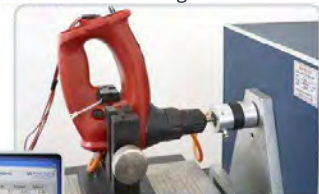
▲ Engine brake - endurance testing
