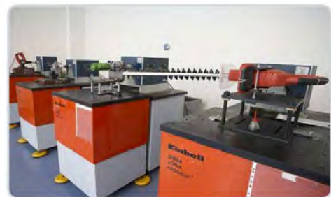
▲ Engine brake - endurance testing
