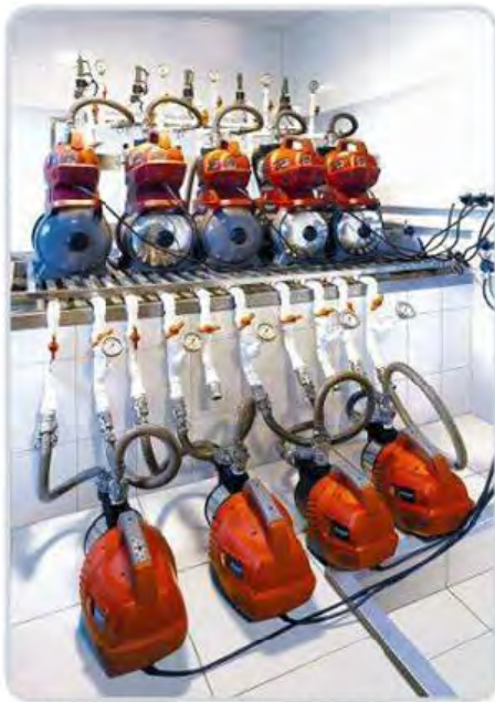
▲ Garden pumps / Domestic waterworks – endurance testing
